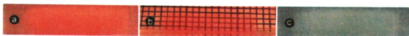
Figure 8. Eosin Yellowish-release from GEPDeN (a) and from hydrogel (b). A blank niosome-containing gel is shown in panel (c). The grid behind the samples is visible only in the sample which does not contain niosomes. These images were obtained after 6 hours.
