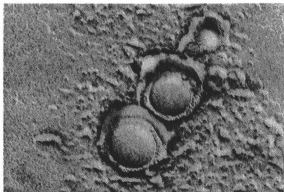
Figure 5. Freeze-fracture electron micrograph of liposomal nanocapsules of about 200 nm in diameter. A thin outer polymer layer that is rougher than expected from a lipid bilayer surrounds the smooth inner lipid membrane.
