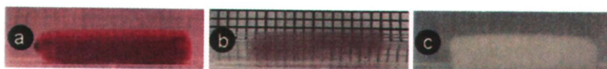
Figure 9. GEPDeN containing Sudan 4, a poorly soluble drug. The drug is only released in niosomes (a), not as free drug (b). As seen in panels (a) and (c), light scattering due to release of niosomes obscures the grid behind the sample.
